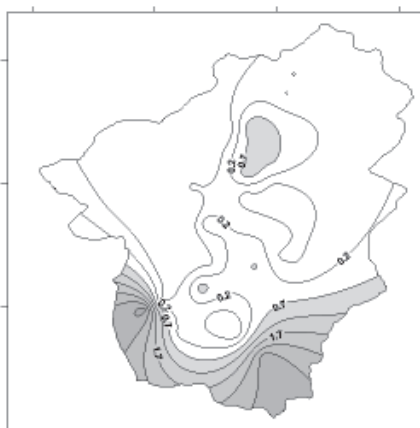
Figure 5. Distribution of Factor score 1 (TDS, Hardness, Mg and Ca) in study area. Area in gray color indicates Factor score > 0.7.
