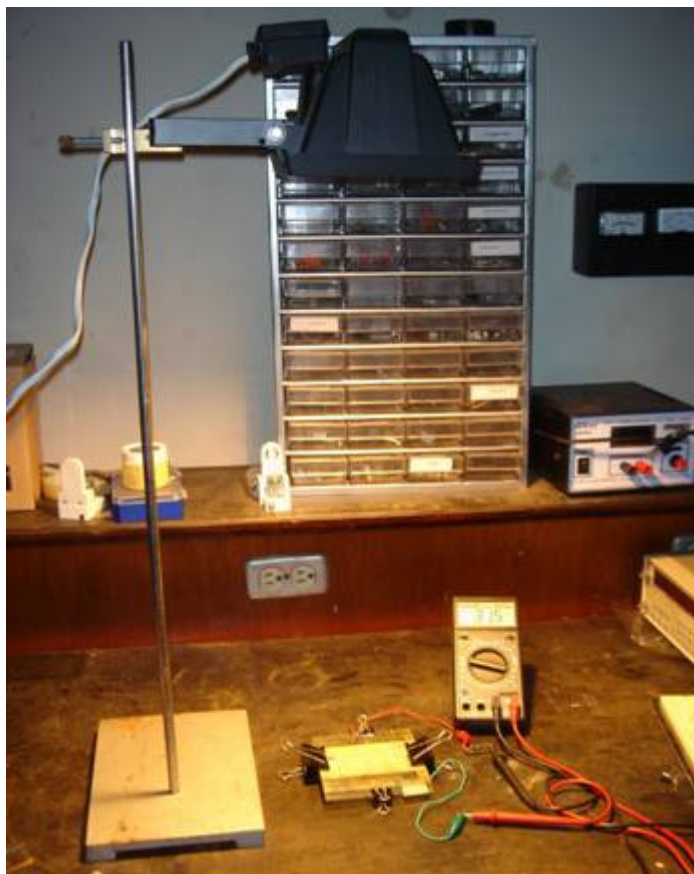
Fig. 1. The experimental set-up for the measurement of photovoltage response of dye-sensitized solar cells on a \text{TiO}_2 electrode with light illumination 1000 lux.
