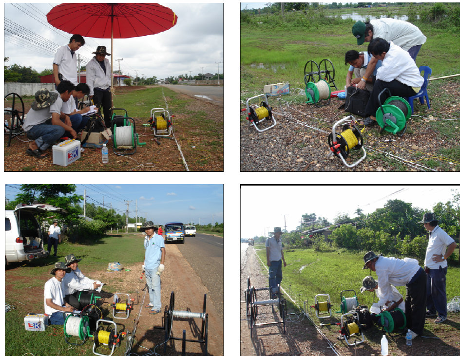
Figure 2.5 Electrical resistivity surveys in Xaithani district
