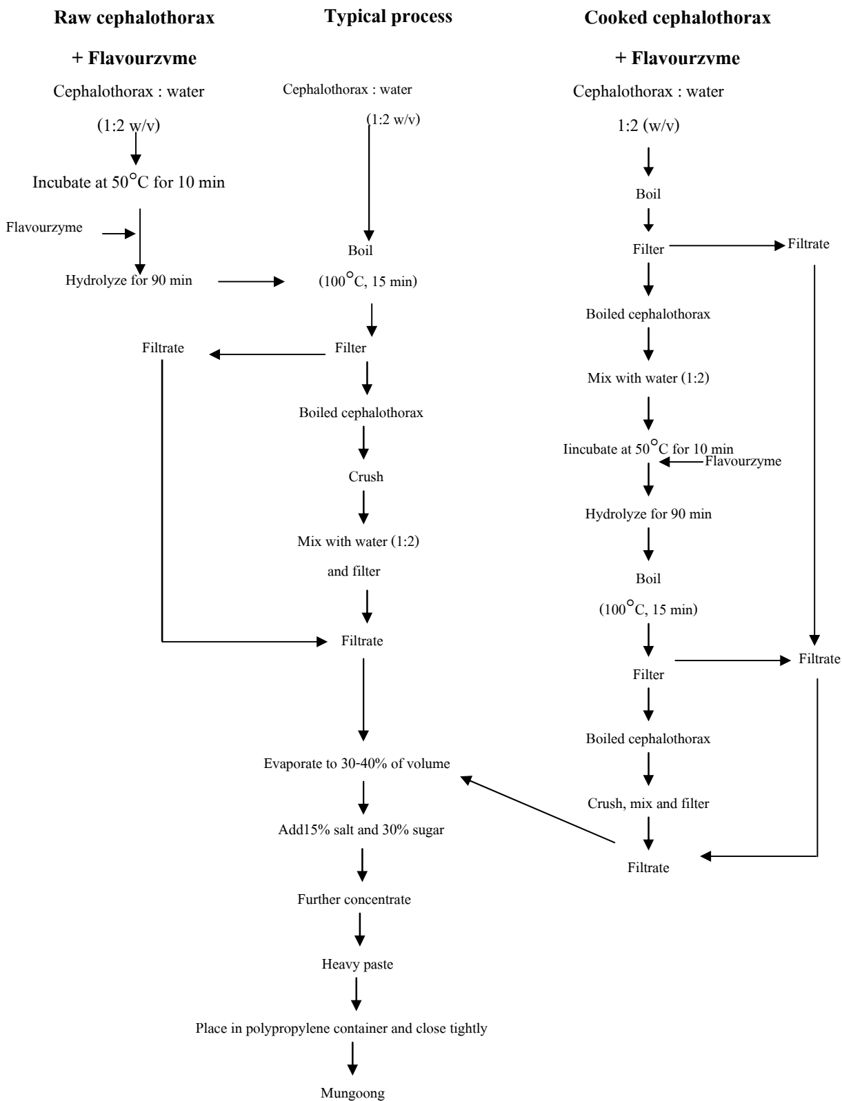
Figure 4 Scheme for Mungoong production
