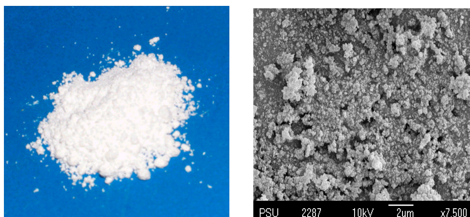
Figure 12 Left: the photograph of commercial TiO 2 Degussa P25 powder (0.1 g) and right: the SEM image of commercial TiO 2 Degussa P25 powder
