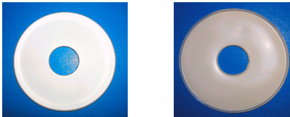
Figure 10 The photographs of Immo-TiO 2 film samples (left: front view ; right : back view)
