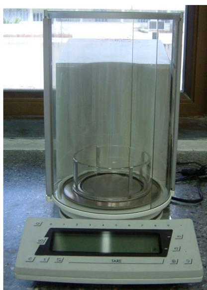
**Fig.24:** Digital scale analytical balance (Sortarius model MC 210S)
