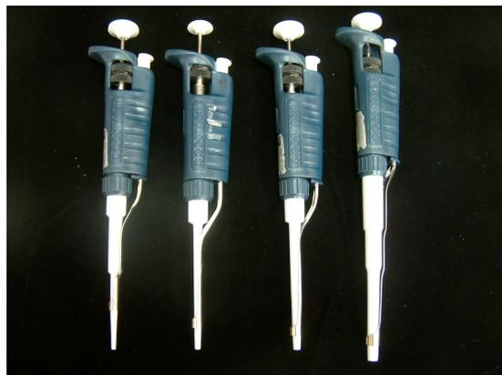
**Fig.23:** Precision pipettors 20, 100, 200 and 1,000  $\mu\text{l}$
