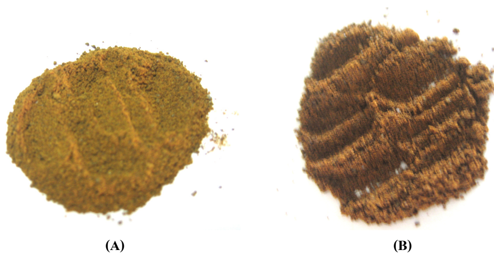
Figure 4.8 Color of the antioxidant active extract of pomegranate fruit peels stored under protected from light (A) and stored under light condition (B) after storage at 45 \pm 2^\circ\text{C}
