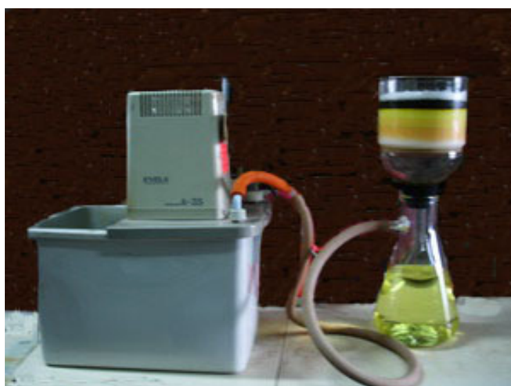
Figure 3-1 Silica gel vacuum column chromatography
