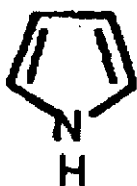
Fig. 2.18. The chemical structure of conducting monomer used to prepare polypyrrole film
