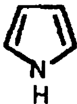
Fig. 5.2. The chemical structure of conducting monomer used to prepare polypyrrole film
