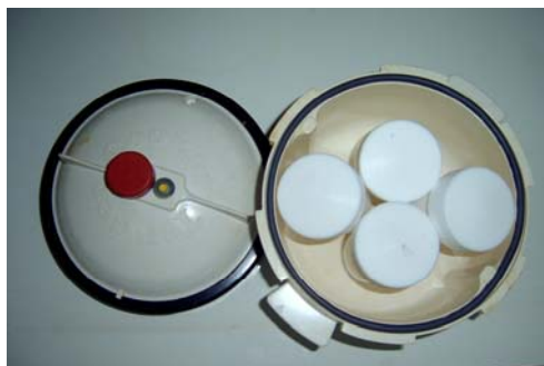
Figure C- 2 The bombs containing the mixtures in a microwave pressure cooker
