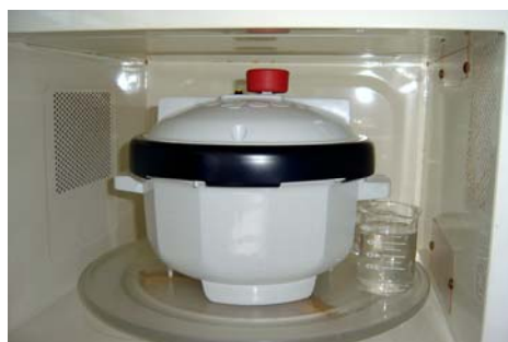
Figure C- 3 The microwave pressure cooker in an unmodified domestic
