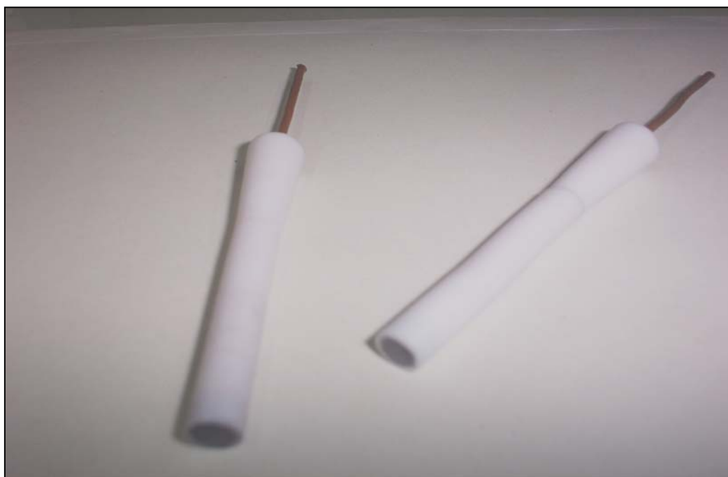
Figure 4 The complete chemically modified carbon paste electrode
