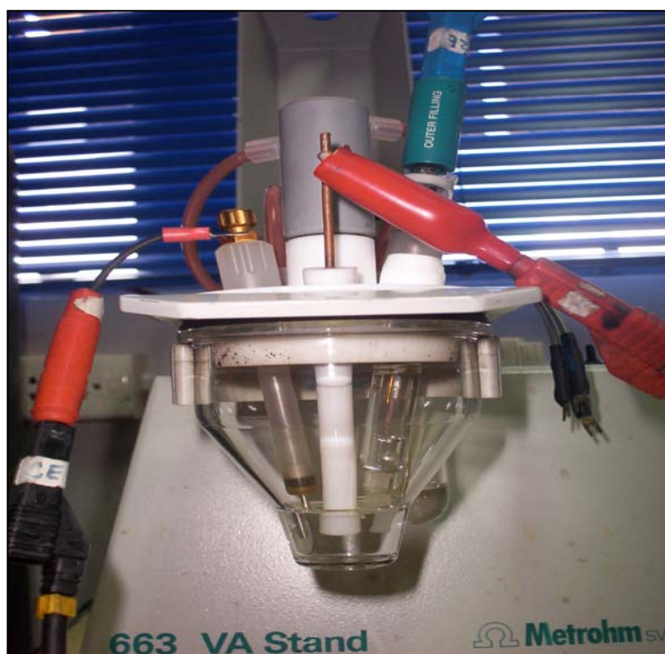
Figure 3 The cell with three electrode system
