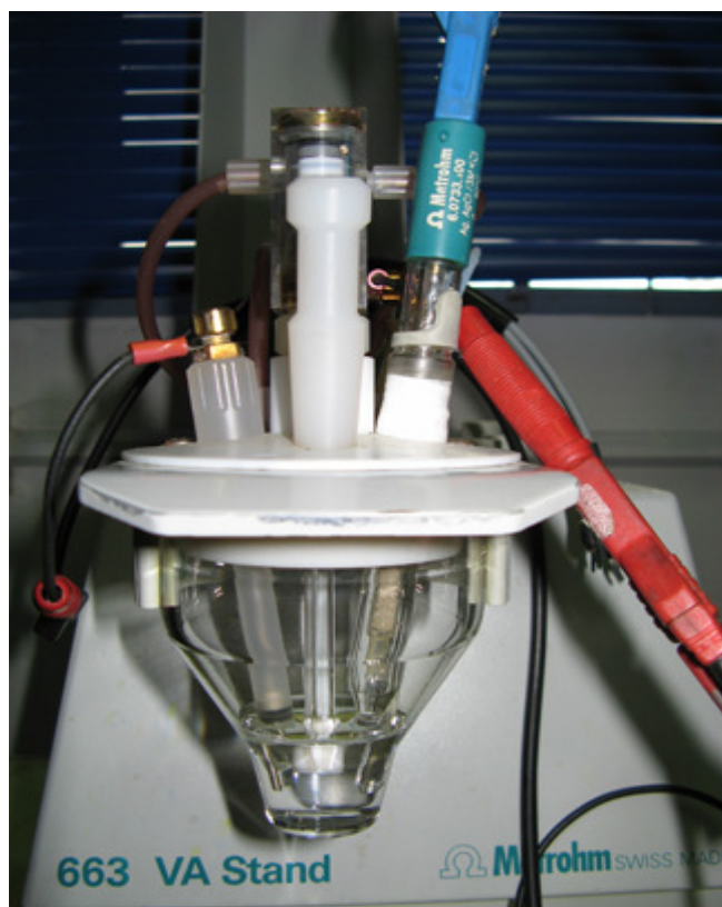
Figure 2-2 The cell with three electrode system
