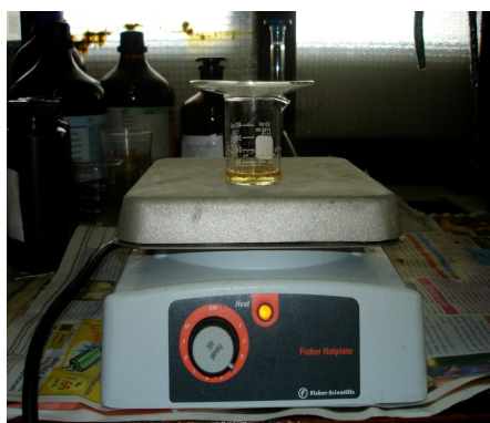
Figure 2-3 Hot plate digestion
