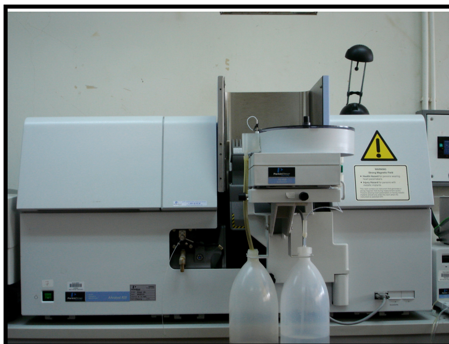
Figure 2-1 Atomic absorption spectrometer (Perkin Elmer Analyst 800 with Zeeman Effect background correction)
