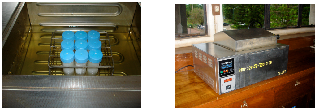
Figure 2-4 Water bath digestion
