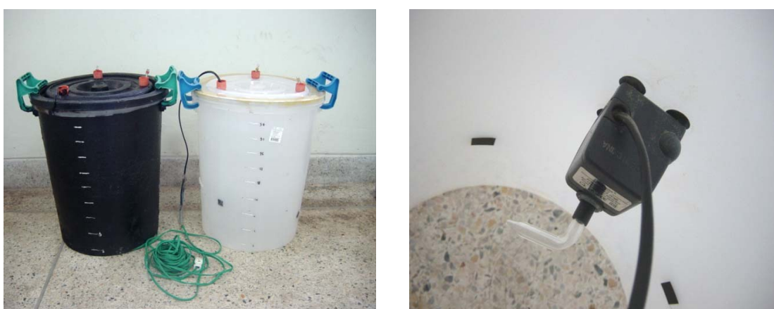
Figure2- 2 Lab-built light and dark benthic chamber (Left) and a submersible pump installed on the wall inside the bucket (Right)
