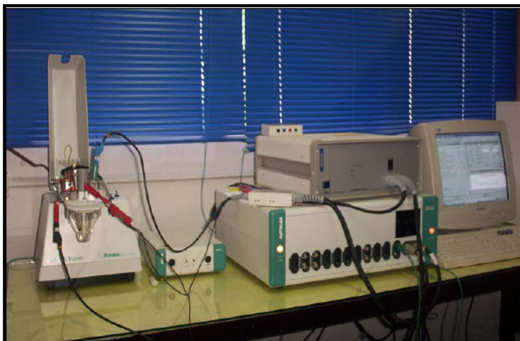
Figure 2-2 Voltammetric equipment (AUTOLAB model PG-STAT 100)
