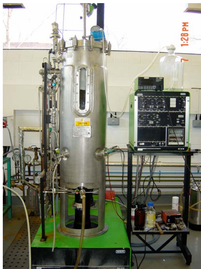
Figure 10.3 Pilot-scale fermenter (150-l) for production of oligodextran
