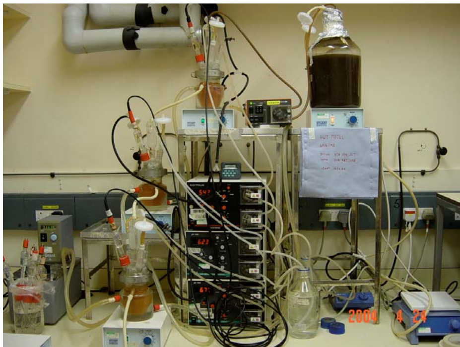
Figure 10.5 Three-stage continuous system (gut model) for fermentation of G19 oligodextran
