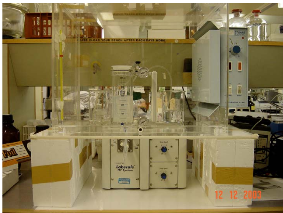
Figure 10.2 Assembly of lab-scale ultrafiltration system
