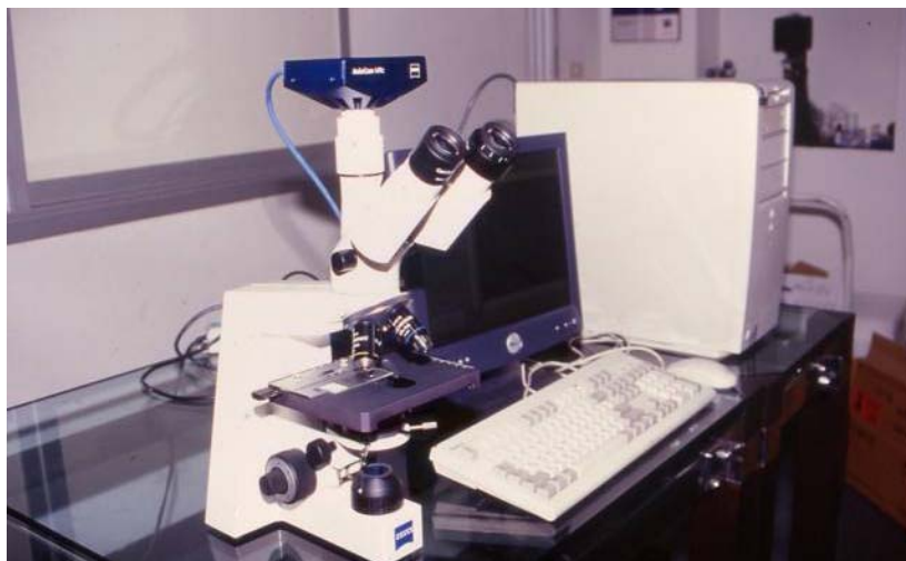
Figure 24. The personal computer, a digital camera (AxioCam MR), light microscope and KS 400 programm were used for histomorphometric analysis.
