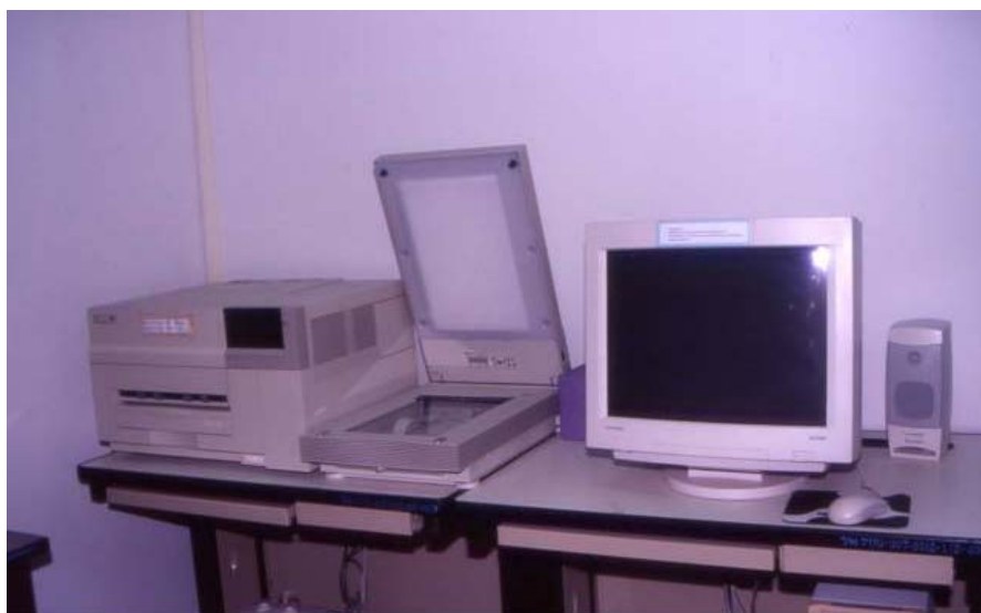
Figure 21. Scanner machine (Scan Jet 4C/T) and computer with Digora analysis soft wear for radiomorphometry analysis.
