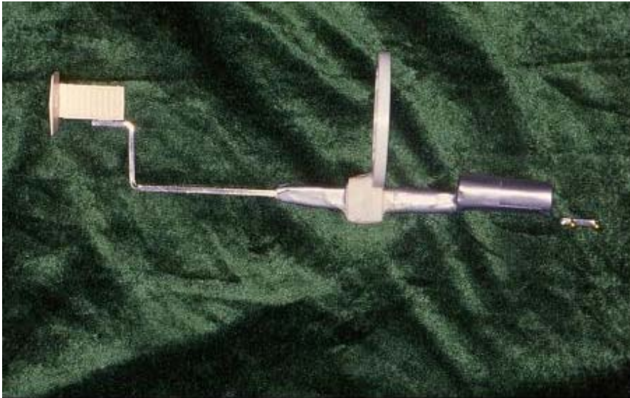
Figure.19. The parallel film holder that developed from XCP. This device is help the researcher to take the radiograph in parallel technique.
