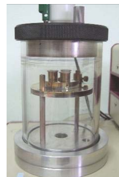
(b) Disk were sputtered coated with gold-palladium particles
