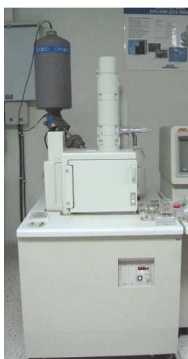
Fig. 12 Demonstrating a gold-palladium coating procedure using a SPI-Module™ Sputter coater (SPI, USA)
