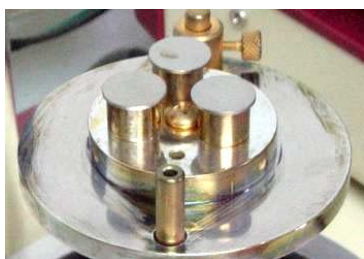
(a) Disks were attached on a stub
