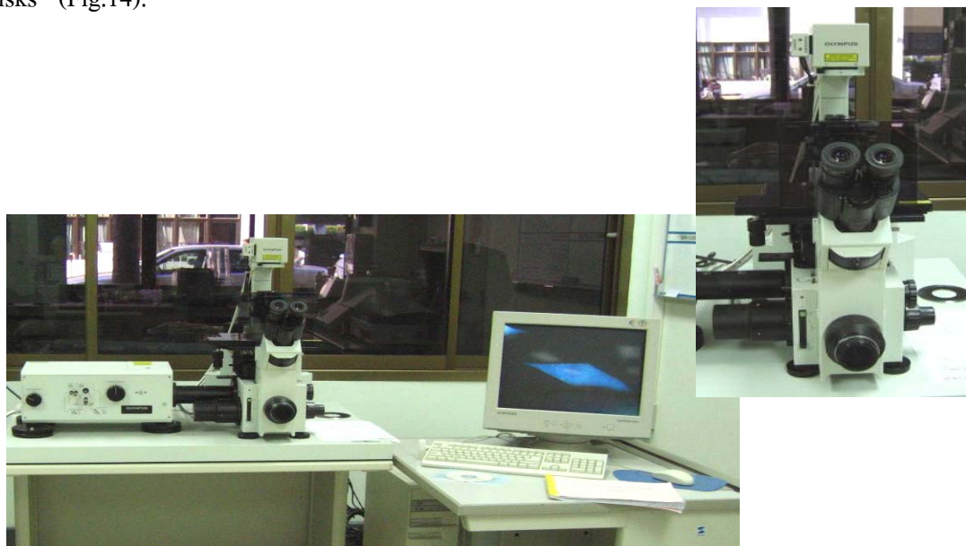
Fig. 14 Demonstrated examing of cells on a titanium disk using CLSM (Olympus FV300 Japan)
