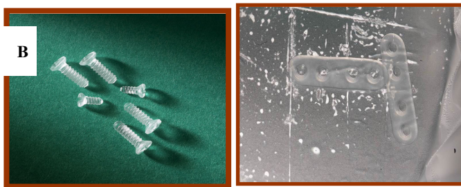
Fig. 6 The resorbable plate, non- self tapping screws.
