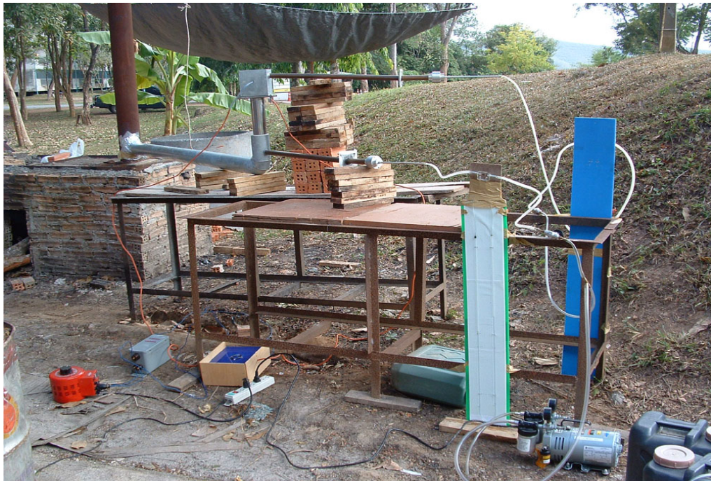
Figure 16. Photograph of the experimental setup for measuring the ESP efficiency on site.
