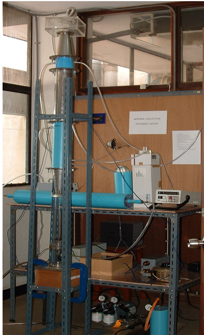
Figure 14. Photograph of the experimental setup for measuring the ESP efficiency in laboratory.
