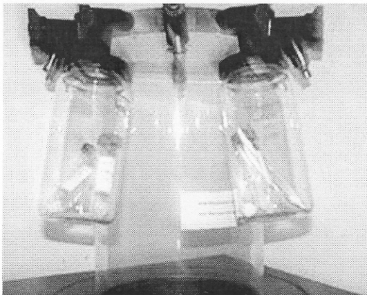
(e) Lyophilization of sterile ICBM scaffold using lyophilizator at -45^{\circ}\text{C} for 12 hours
