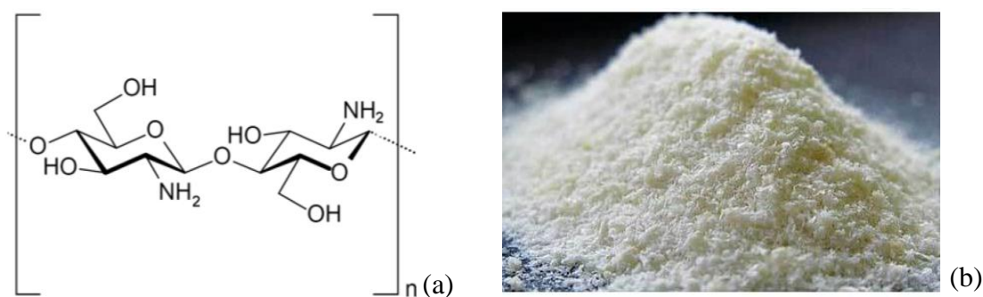
Figure 2-9 The chemical structure (a) and physical appearance (b) of chitosan
