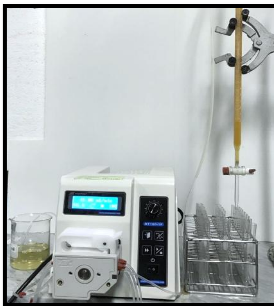
Figure 60 Column adsorption of lactic acid from fermentation broth
