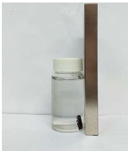
Fig. A1.2.7 Neodymium magnet grade N35 (100 mm x 50 mm x 10 mm)
