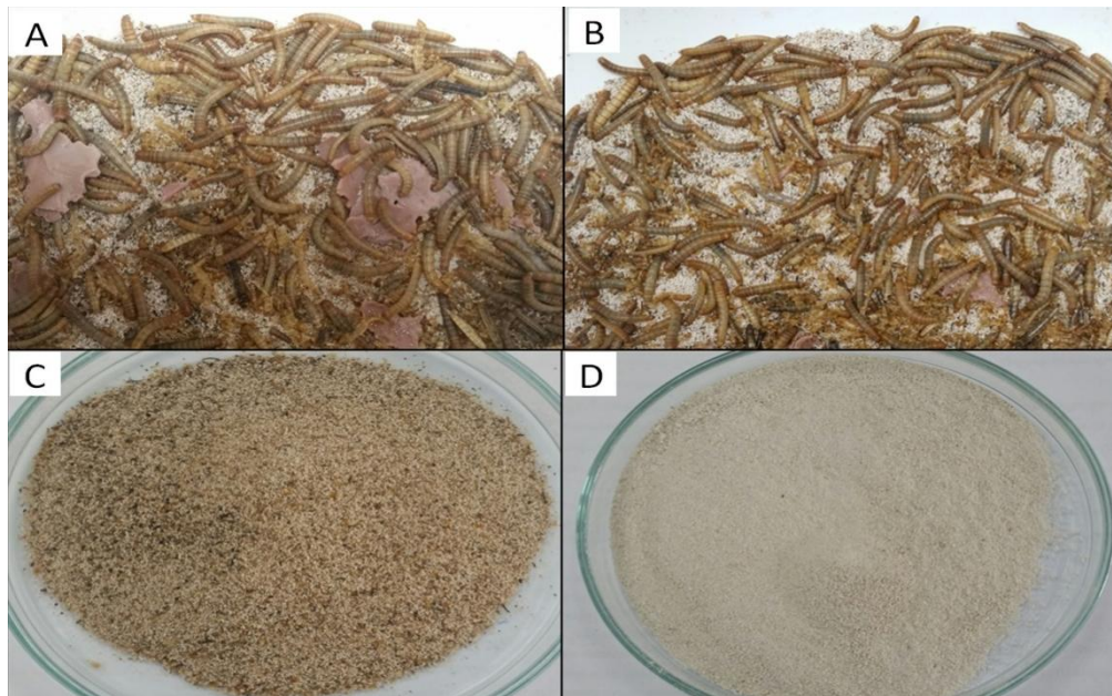
Figure 24 Biological recovery process of PHAs from P. mendocina PSU cells using mealworms. ( A) Mealworms feeding on dried P. mendocina PSU cells (B) Mealworms and fecal pellets after almost complete feeding on cells (C) Fecal pellets before washing and further purification (D) Fecal pellets containing PHB after being purified by 1% SDS
