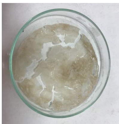
Figure 25 PHB was blended with modified ENR25 rubber (70:30) by solution Blending (chloroform)
