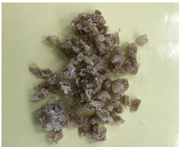
Figure 27 PHB was blended with modified ENR25 rubber (70:30) by twin screw extrusion
