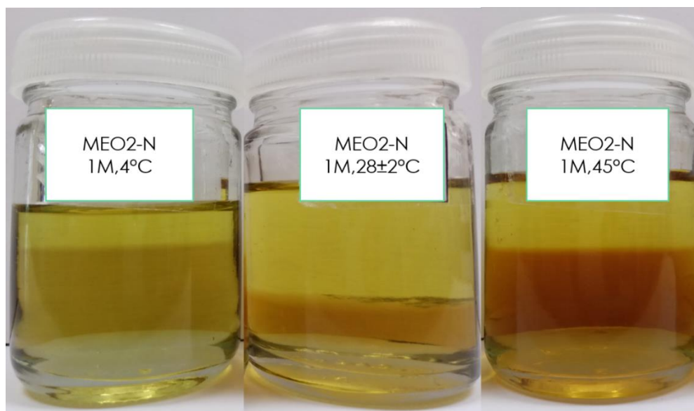
Figure 24. Physical appearance of MEO2-N at the first month stored at 4°C, room temperature ( 28 \pm 2^\circ\text{C} ) and 45°C.
