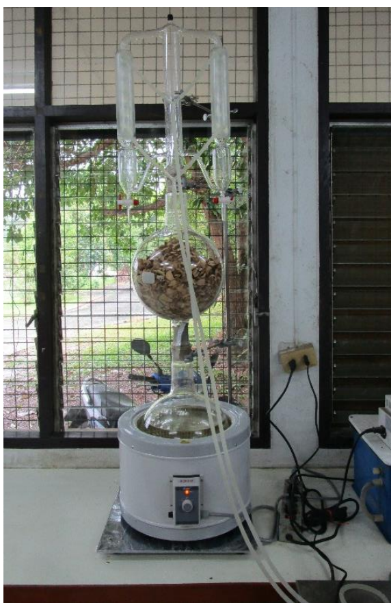
Figure 4 Clevenger type apparatus for extracting essential oil by steam distillation.
