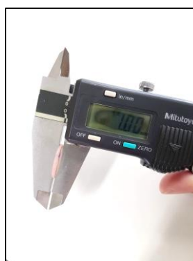
Figure 7 Verification of the root section thickness by digital caliper
