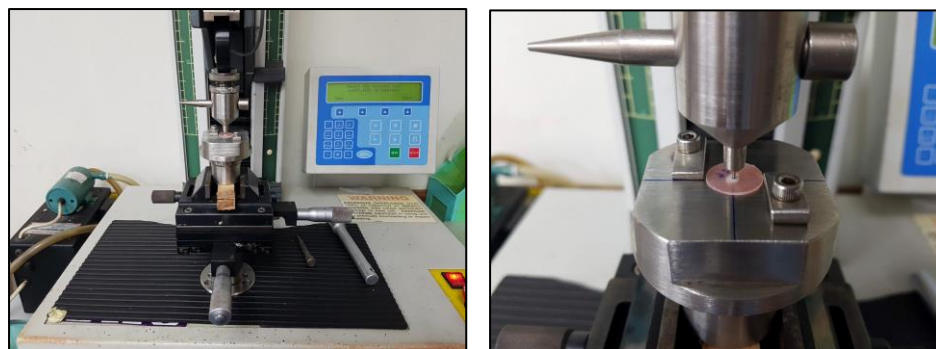
Figure 9 Universal testing machine's setting for push-out testing
