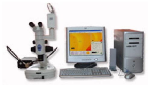
Figure 11 Stereoscopic microscope using in radius measuring and failure determining
