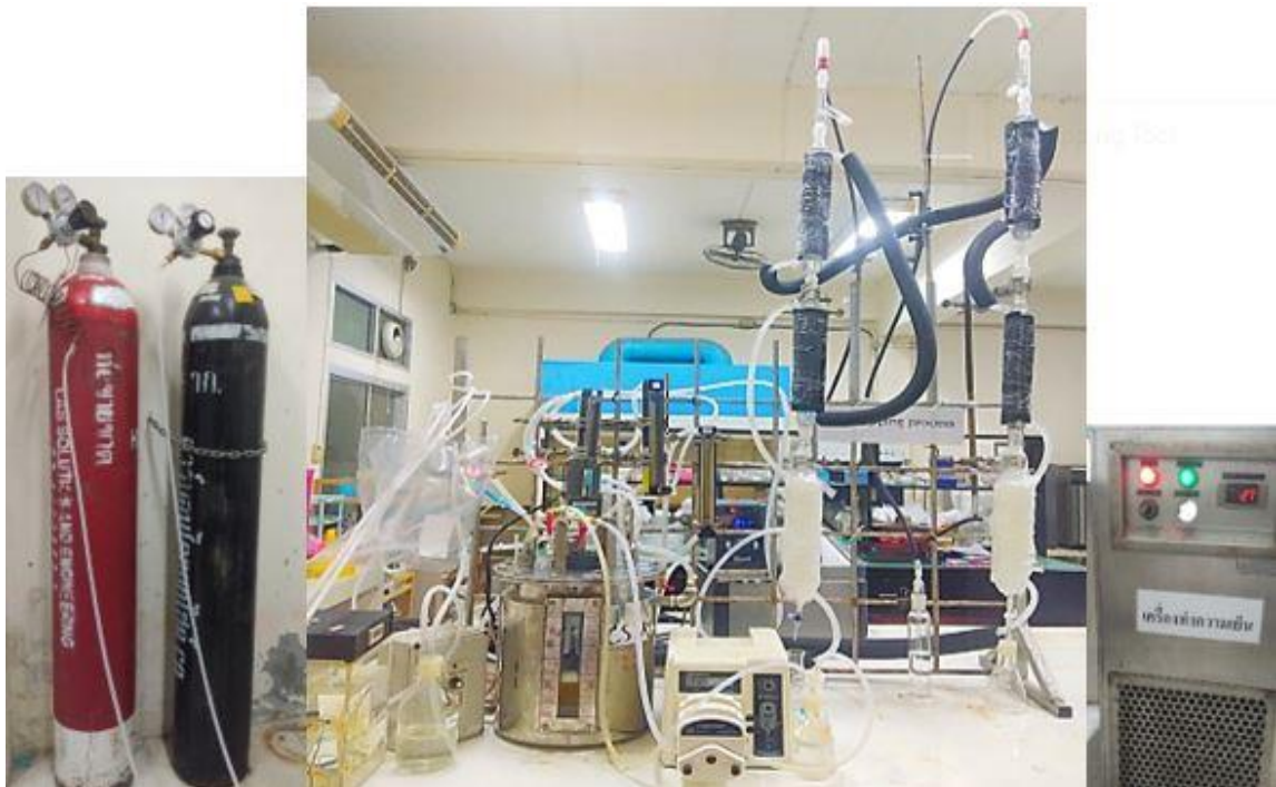
Figure 33. Second CSTR system for butanol production equip with gas stripping process.
