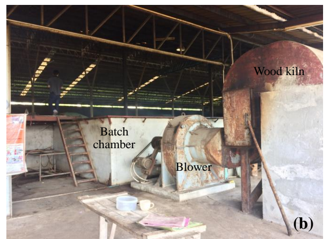
69 70 Fig. 2. The photos of industrial batch drier (a) the top of batch chamber and (b) hot air 71 supplier.
