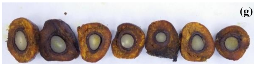
Fig. 9. Visual appearance of internal dried palm fruit in different drying time at (a) 8 hours (b) 14 hours (c) 18 hours (d) 20 hours (e) 22 hours (f) 24 hours and (g) 26 hours (continued).
