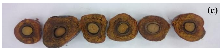
Fig. 10. Visual appearance of internal dried palm fruit in different position of (a) upper of batch dryer (b) half height of batch dryer and (c) bottom of batch dryer.
