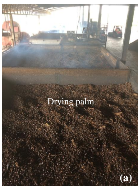
69 70 Fig. 2. The photos of industrial batch drier (a) the top of batch chamber and (b) hot air 71 supplier.
