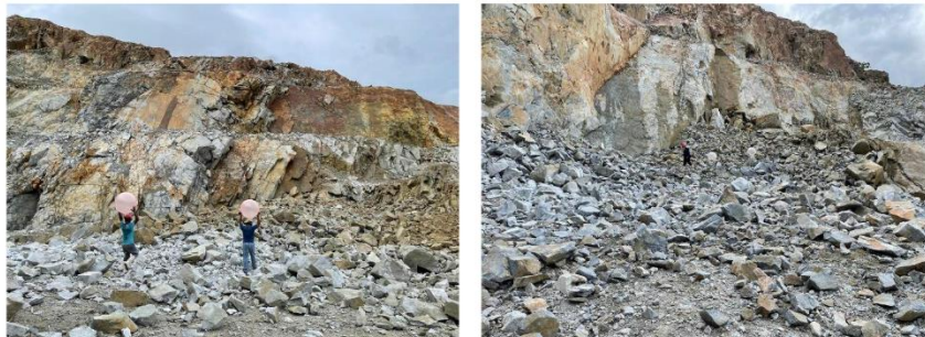
Fig. 9 Pile of rocks after the blast.
