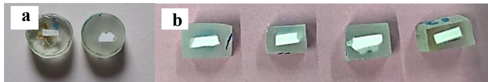
Fig. 3.3 Sample of K0, K4, K8 and K12 (a)-(b) Before and after sandpaper polishing.
