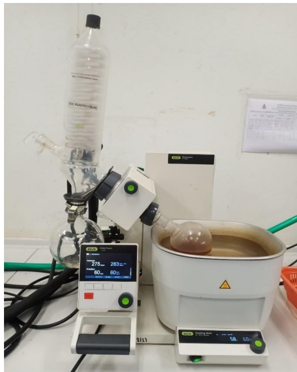
Figure 3.5 Methanol recovery process with a rotary evaporator
