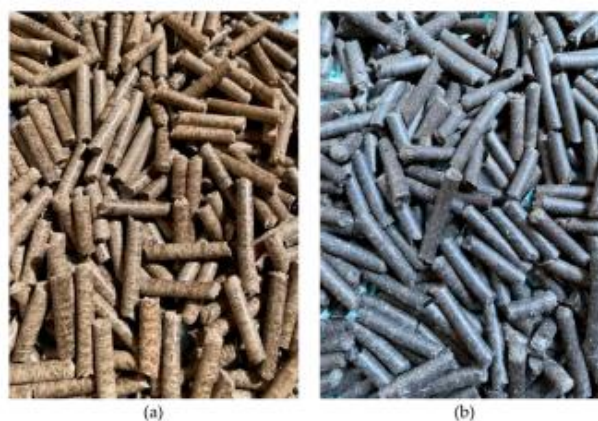
Figure 3. Visual appearance of (a) rubberwood pellets and (b) mixed pellets, i.e., 50% rubberwood and 50% RDF.
