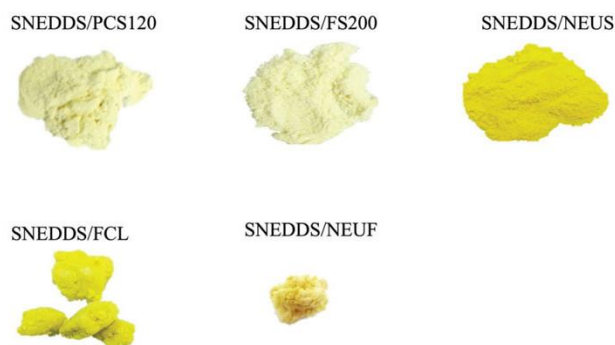
Figure 1. S-NEDDS formulations prepared by adsorption of SNEDDS onto solid carriers. (i.e. FS200, PCS120, NEUS, FCL, and NEUF).
