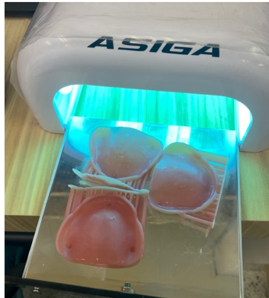
Figure 11 light cured 3D-printed denture for final polymerization
