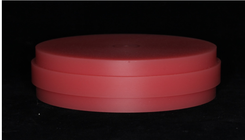
Figure 7 Prepolymerized polymethyl methacrylate block for milling
