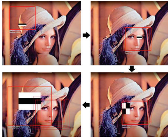
Figure 20. Demonstrate the work of the Haar Cascade.
