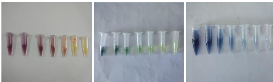
Figure 41. Antioxidant assay (a) DPPH assay with trolox standard (7.8125-500 mg/L) (b) ABTS assay with trolox standard (7.8125-500 mg/L) (c) FRAP assay with FeSO 4 standard (0.1-1 mM)
