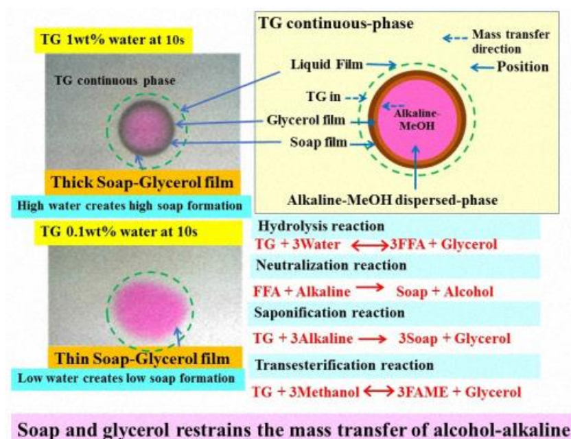
Fig. 3.6 The possible model of reaction zone for the effect of water on RPO saponification with initial excess RPO
