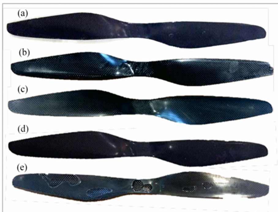
FIGURE 8 Top views of the UAV blades produced from eco-nanocomposites of epoxy resin with 3 phr ENR 50 and various nanosilica amounts (0, 1, 2, 3 and 4 phr); by (a) without nanosilica, (b) 1 phr nanosilica, (c) 2 phr nanosilica, (d) 3 phr nanosilica, and (e) 4 phr nanosilica
