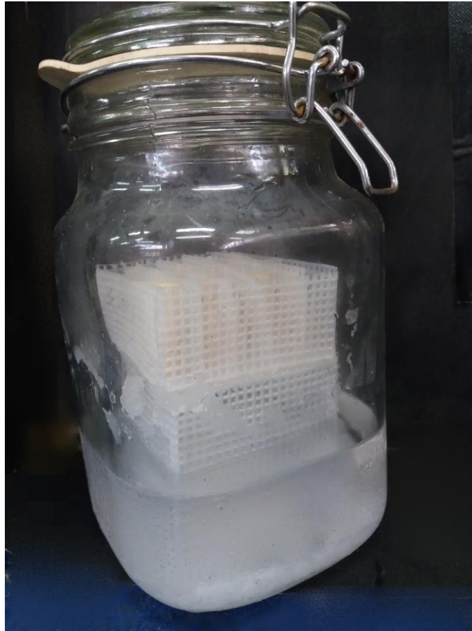
Fig. 2-5 Experimental apparatus for the sorption isotherms measurement.
