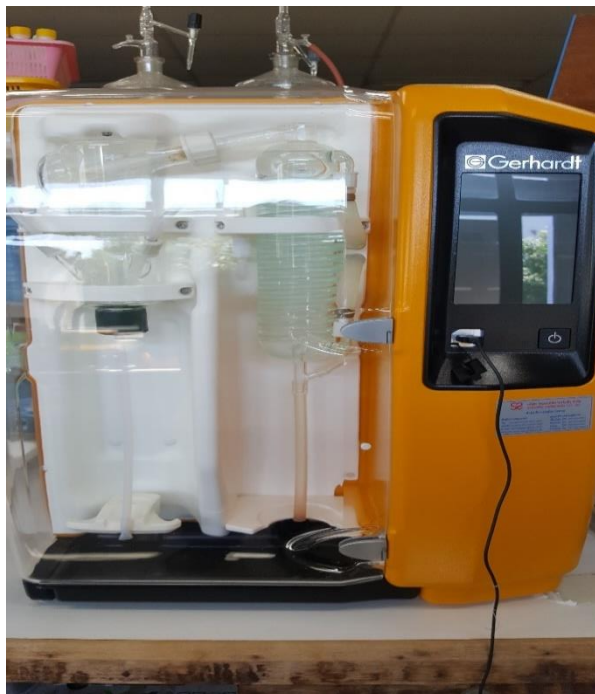
Figure 3. 6 Gerhardts (Germany) ammonia distiller to calculate CEC
