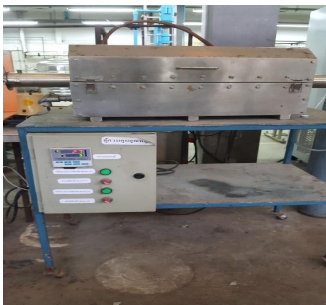
Figure 3. 3 Pyrolysis process a) tubular reactor b) heating box with coils c) Temperature controller (3 cycle)
