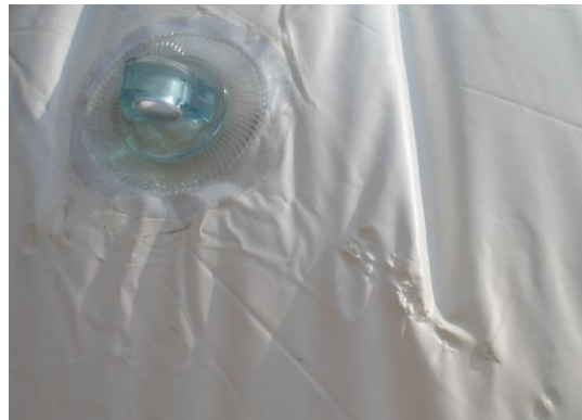
12. Damage caused by transportation (This is the second balloon)
