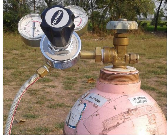
2. Install a regulator to helium tank
