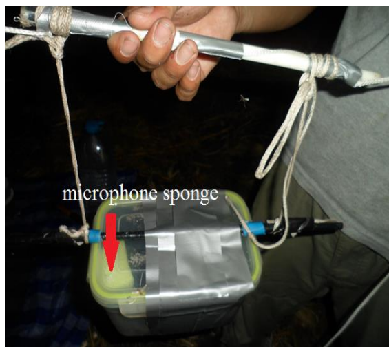
1. A box contains bat detector and recorder
