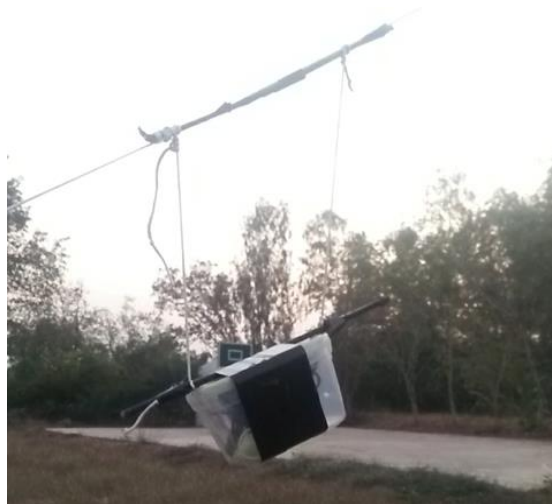
2. The box is mounted to the balloon line
