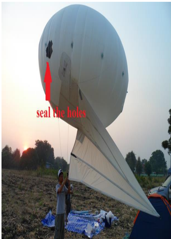
13. Luckily, we could seal the holes and continued the campaign
