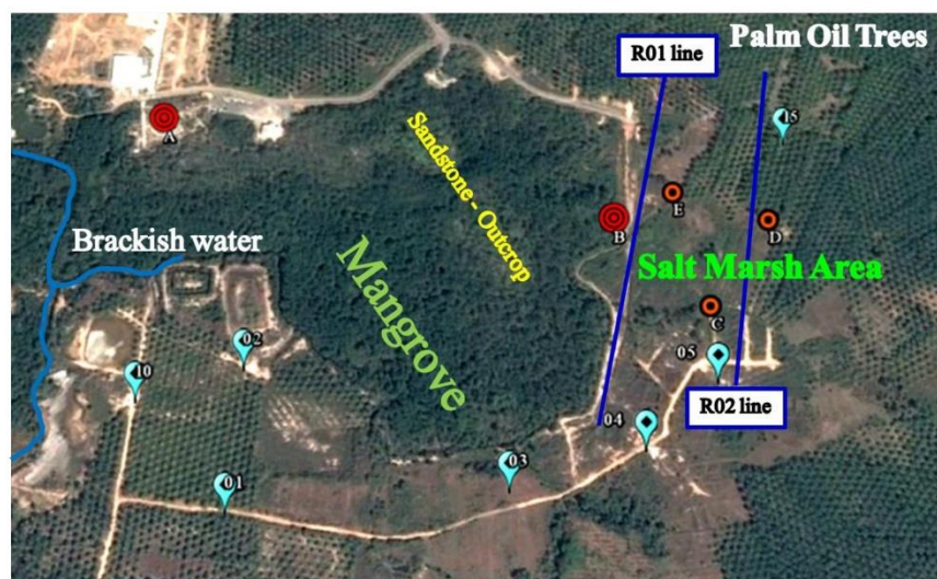
Figure 2: Location of natural hot spring, local wells (A: KB4/5; B: KB4/10; C: Well01; D: Well02; E: Well03) and geophysical survey locations, with number from 1-15 (not all shown on the map) indicate VES points, and R01 and R02 indicate ERT lines.
