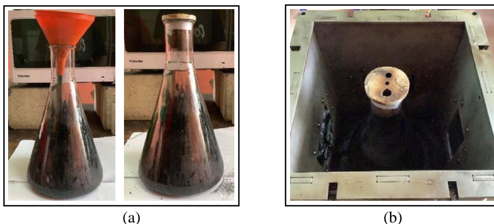
Figure 3.5 (a) Packing of test material in quartz reactor (b) filling the quartz reactor in the microwave (cavity)
