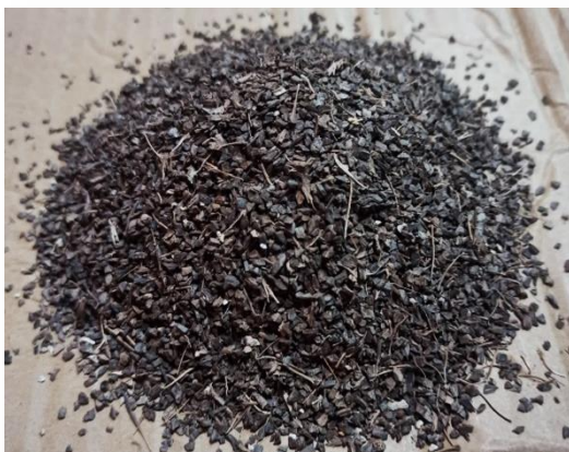
Figure A2 Physical characteristics of OPS after grinding.
