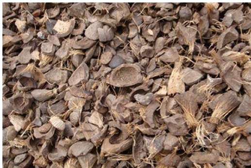
Figure A1 Physical characteristics of OPS before grinding.
