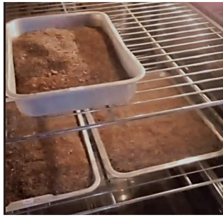
Figure A5 Raw materials dried in a hot air oven at 105 °C.
