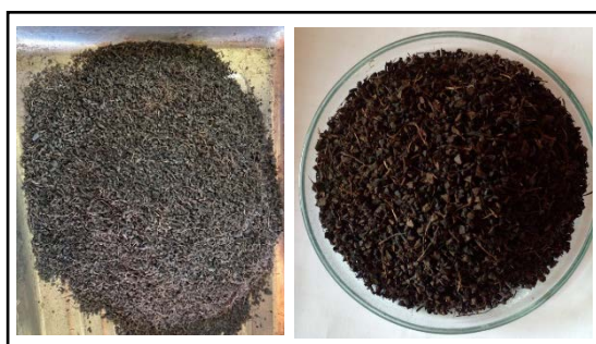
Figure 4.7 Solid product (bio-char) obtained by microwave pyrolysis.
