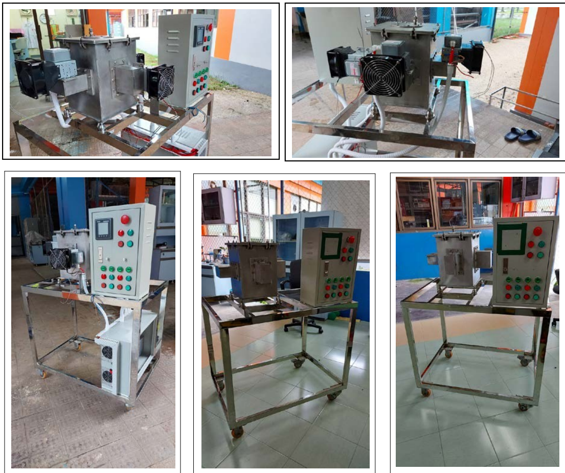
Figure 4.4 Prototype microwave pyrolysis system for producing crude bio-oil and bio-char
