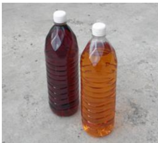
Fig. 1. 4 Bottles of non-distilled (left) and distilled (right) mangrove pyrolysis liquid (Chan et al., 2012)
