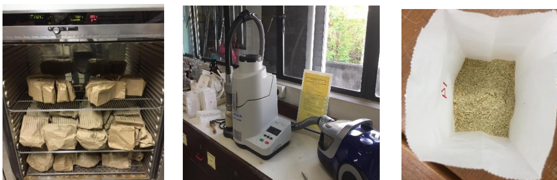
Figure 4. Plant biomass samples drying, preparation and grinding in grinder model: Retch Cyclone Mill Twister.
