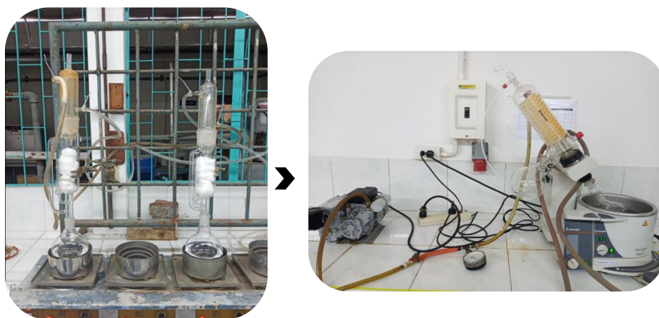
Figure 2.8 Oil content analysis by Soxhlet and Rotary evaporator.
