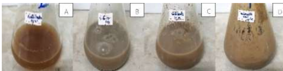
Figure 15 Sample sources from tuna canning industry for isolation of lipase and protease producing (EM for smell reduction (A), sludge from microorganisms collecting sludge pond (B), wastewater from oil trap (C), and scum from oil trap (D)).
